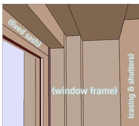
Fig. 5: Reconstruction drawing of the upper inside corner of window OPL\_007, showing (at left) a fixed sash for the mounting of glass window panes 0.003m thick.
